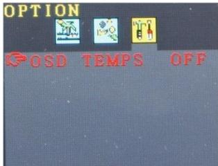
The 'Option' submenu allows activating a function ensuring the screen menu is switched off automatically.
