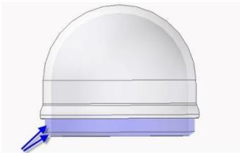
Before fitting the new dome, lubricate the threading with silicon. When changing the dome, check it is screwed tight until the last screw pitch. Otherwise, the sealing of the camera head is not guaranteed and its operation may be disturbed by penetration of water or dirt.
