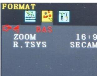
The 'Format' submenu allows rotating the screen display, modifying the screen format from 16:9 to 4:3 or selecting the video format.
