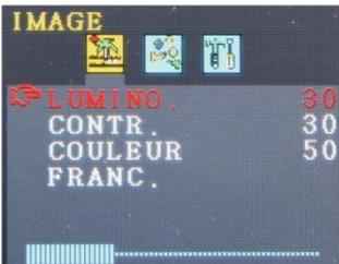
The 'Image' submenu allows setting the brightness, contrast, and colour between 0 and 100.
