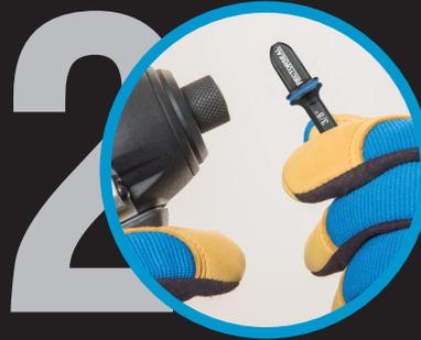
Choose bit size & attach it to the chuck or coupler. Fasten it well. Set power tool to MAX speed & torque if it is adjustable. Check power tool is not in hammer mode.
