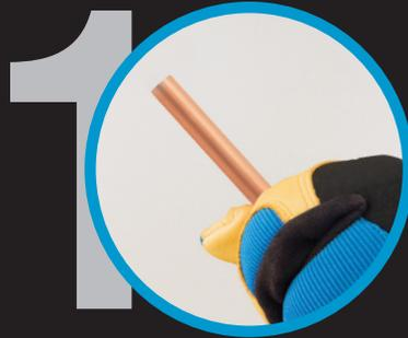
Firmly hold tubing at all times. Keep a safe distance between your hand and the tube's border.
