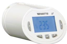
Programmable electronic thermostatic head for radiators. Can either be used as a stand-alone device (9 pre-set and 4 customisable programmes) or in conjunction with the WATTS® Vision® central control unit (**BT-CT02 RF/WiFi Series**) and **BT02-RF Series** thermostats.
