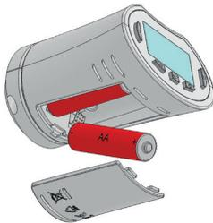
**Note:** The batteries can be changed with the head installed.
